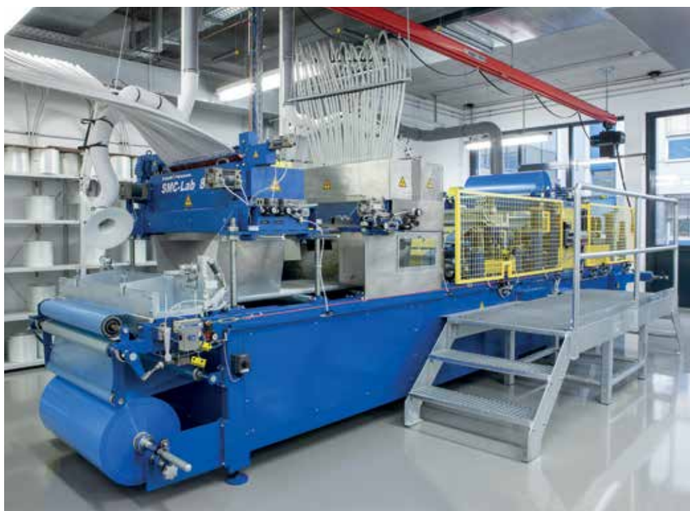
SMC Line with Glass and Carbon Fiber Cutting System
