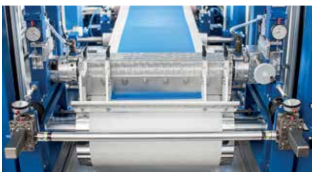
Coating Head with Optional Viscosity Measurement
