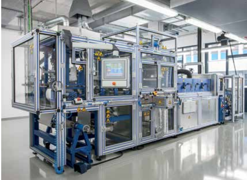
Spread Coating Line with Gelling Drums, Oven and Lamination Facility
