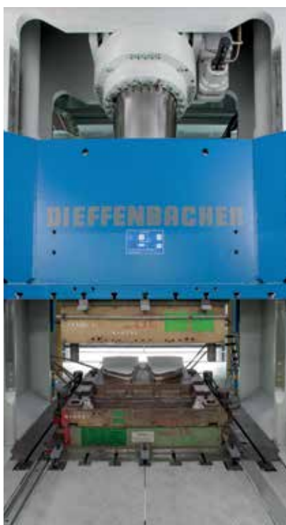
Compress Eco with a Maximum of 1,000 Tons of Press Force
