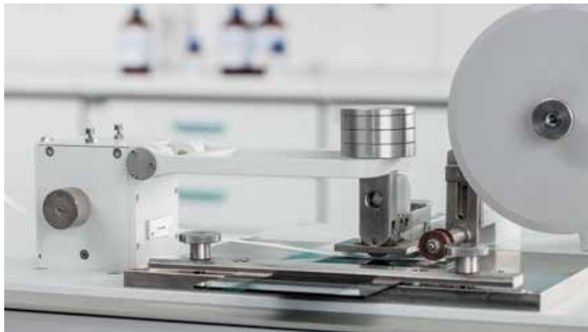
Abrasion Testing with the Wazau Device
