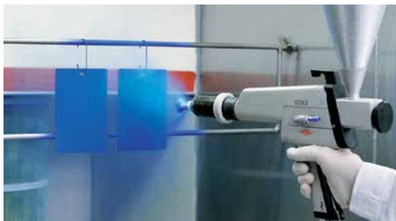
Application Using a Powder Spray Gun
