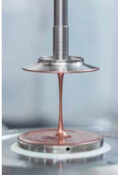
The Rheometer Tests the Flow Behavior
