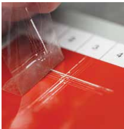
Cross-cut Test to Determine Adhesion
