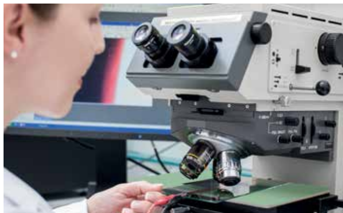
Pigment Charge Measurement under the Microscope
