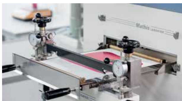
Laboratory Dryer with Coating Unit
