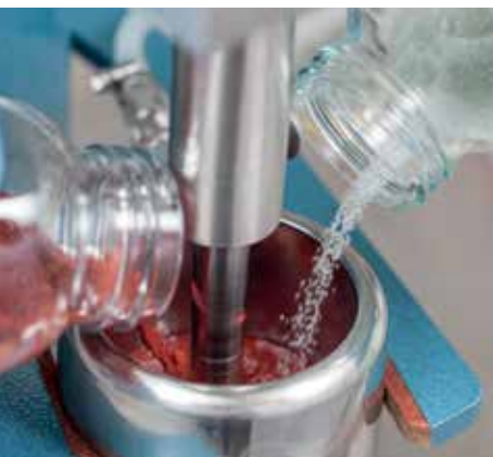
Pigment Grinding with the Dispermat
