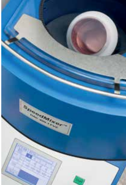
The Speed Mixer Creates Adhesive Specimens
