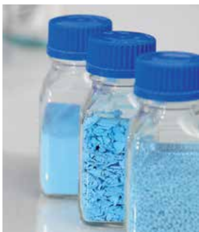
Raw Materials Mix: Powder Coating Chips and the Resulting Coating after Grinding
