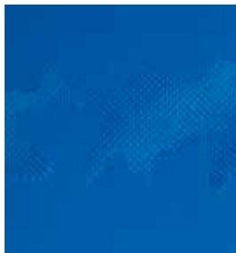
Poor substrate wetting of an aqueous coating on PVC foil
